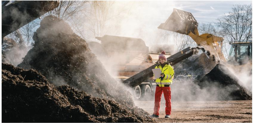
The material is placed in large piles, where microorganisms begin to break it down and heat up the piles to very high temperatures.
